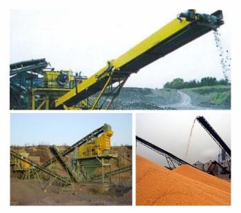
The conveyor can be divided into two types: the lifting type and the non lifting type, the conveyor belt is driven by the electric roller, the lifting and running of the whole machine is non motorized, if need, can be designed as motorized or electric.
